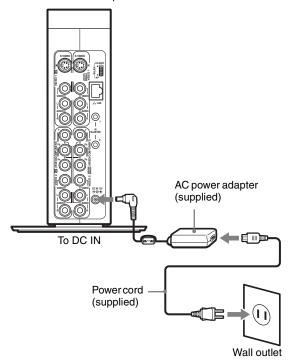
Connect the power cord to the Base Station AC power adapter, and the AC power adapter to the DC IN jack on the Base Station, then plug the power cord into a wall outlet.
